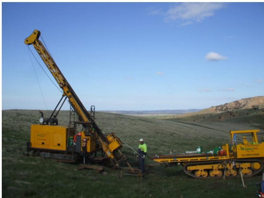
Figure 1: Diamond drilling the Eastern Side of the Princess Royal looking South East
